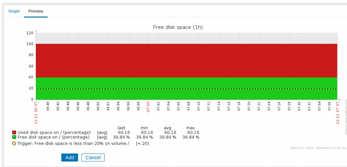
In this example, pay attention to the dashed bold line displaying the trigger level and the trigger information displayed in the legend.
