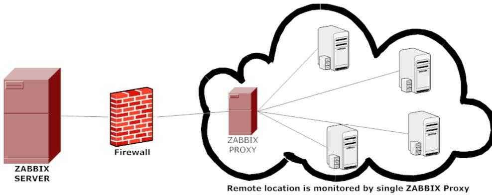
The proxy requires only one TCP connection to the Zabbix server. This way it is easier to get around a firewall as you only need to configure one firewall rule.
